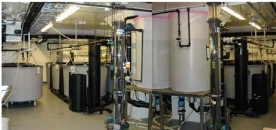
The experiment examined the microbial communities within a flow-through system and recirculation systems with ozone or ultraviolet treatments.
